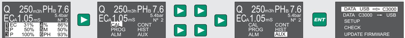
Option to load the Configuration and Programming from a pendrive.
