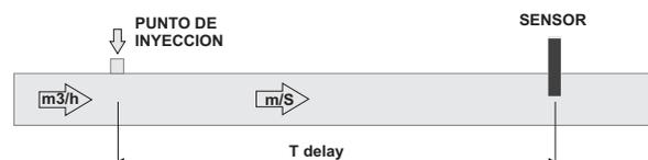
**Tdelay delay time of channel A:** It is the time lightly bigger than the necessary time since a product has been injected into the tubes, until this one comes to the corresponding sensor (EC or pH), with a certain flow ( $Q_{test}$ ).
