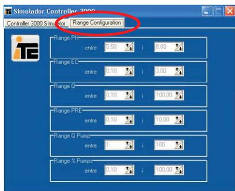
Configuration of the limits of the random values generated for pH, conductivity, flow, pressure, pumps, and dosage percentage. This screen is only valid when the Auto option is activated.
