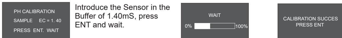
Validate the EC Calibration by pressing ENTER.
