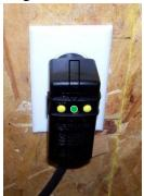
This Germination chamber is protected with a GFCI equipped cord. If the digital display does not come on when the cord is plugged in check that the reset button is set and the green light is on. Once the cord is plugged in the digital display on the thermostat will cycle through its startup routine. If the display does not come on check to make sure there is power at the plug and that the reset button has been pressed. Unplug the germination chamber for storage or to turn off the thermostat.
