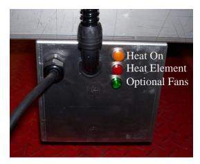
If the Germination Chamber does not seem to come on after it is plugged in make sure the water reservoir is full, the GFCI cord end shows a green light and the digital display, on the thermostat, is working. Finally make sure that the room the chamber is located in is not hotter than the "turn on" temperature for the heater.
