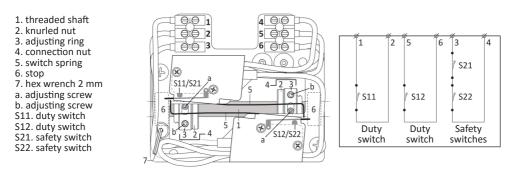
The following information explains the working and setting of the limit switch system. **Current (I) in the switching circuit at 24 V AC:**
