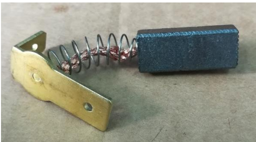
Figure 5d: Inspecting the carbon brushes
