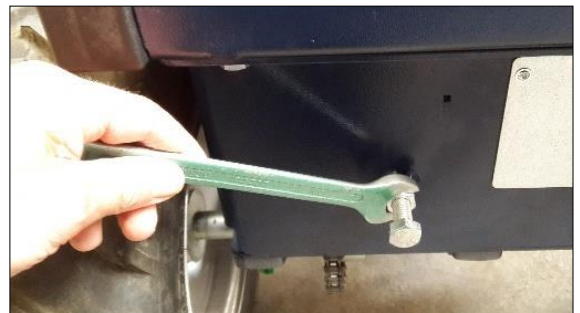
Figure 9: Loosen/tighten the locking nut
