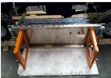
Take a platform (Package B), lay it on a piece of cardboard and unscrew the bolts.
