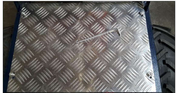
Figure 7: Dismantle the checker plate
