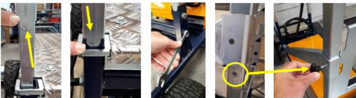
Mount the four uprights and tighten the eight bolts using a 17 mm spanner, while noting the notches indicated, there is one upright with a threaded hole, this one should be mounted at the drive wheels.
