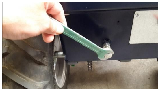
Figure 10: Tension the chain
