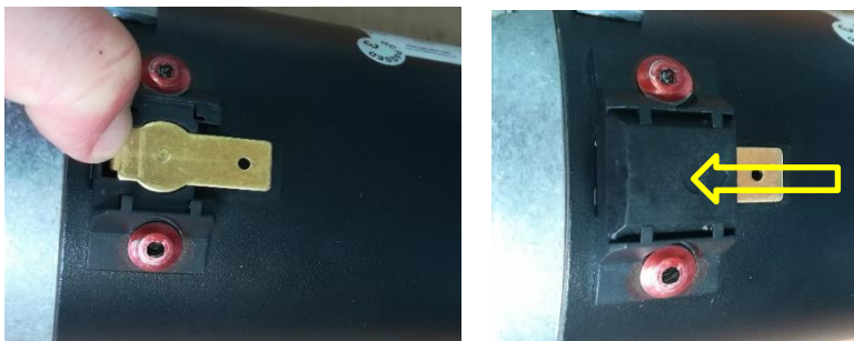
Figures 5d & e: Mounting the carbon brushes
