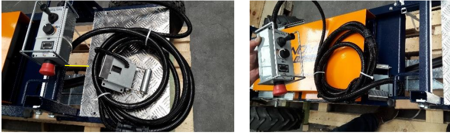
Cut off the cable ties and pull the cabling under the tubular frame.
