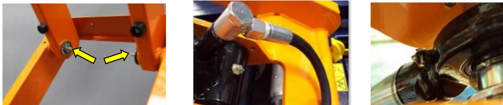
Figure 9.3; Location of the grease nipples at the cylinder
