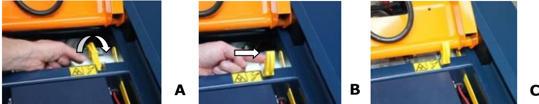
Figure 9.1 A-B-C; Unlocking the scissor blocks
