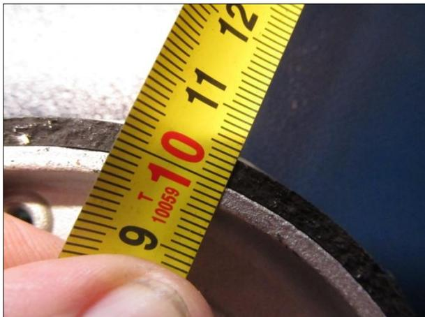
Figure 11: Measure brake shoe lining
