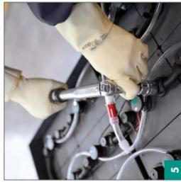
Check that all screws are tight, especially on the battery terminals:
