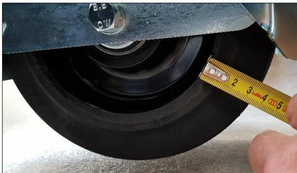
Figure 15: Check for wear, measure example
