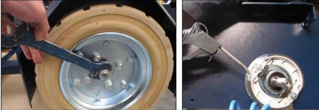
Figure 11: Disassemble wheels
