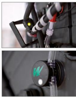
When necessary, top up the battery with distilled water, when charging is complete.
