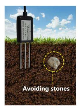
**Buried measurement**: Vertically dig pits with a diameter of >20cm, insert the sensor steel needle horizontally into the pit wall at a given depth, fill the pits tightly, and stabilize for a period of time, then measure and record for several days, months or even longer.
