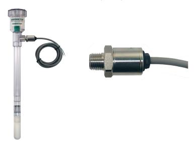
**The IRROMETER RSU-C** is a pressure transducer sealed in a stainless steel housing, which converts the 0 to 100 kPa tension reading from the instrument into a 4-20mA current output. Any device which can read a 4-20mA sensor and can supply between 9 and 36VDC can read the RSU-C.
