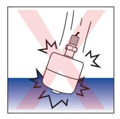
**Handle With Care** Avoid dropping float. Could effect sensor
