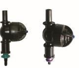
Super LPD is the latest Leakage Prevention Device for use for the greenhouse micro sprinklers. The Super LPD allows micro sprinklers to start-up and shut-down simultaneously. Its check valve function eliminates water damage by preventing leaks after the system shut-down. Available in High and Low pressure models. Made of three parts for simple maintenance.
