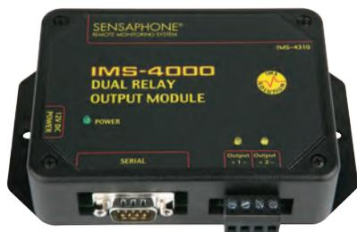
The IMS-4310 Dual Relay Output Module allows you to control two devices from any IMS-4000 Host or Node. Each output may be controlled either manually or automatically. Each output has the option of providing either a dry relay contact or 12VDC power. Two switches located inside the device select the output type.
