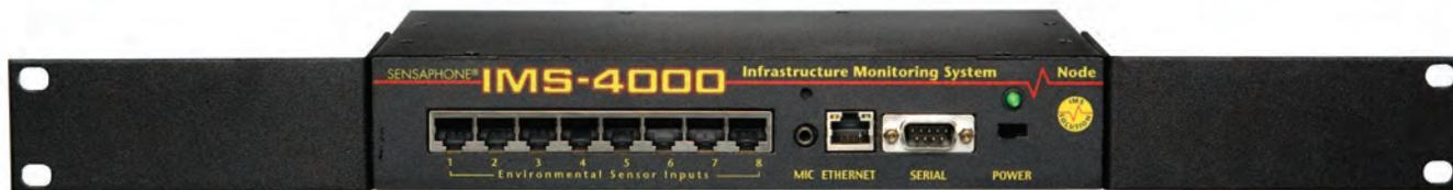
The IMS-4000 Node allows IMS-4000 users to expand their infrastructure and monitor additional inputs in locations away from the IMS-4000 Host. Up to thirty-one Nodes can be used with each IMS-4000 Host. Much like the Host, the Node can monitor eight inputs for environmental conditions and or alarm contacts from other computer equipment such as UPS systems. The Node connects to the Host via a RJ-45 10/100BASE-T Ethernet and is monitored via the ConsoleView software included with the Host.
