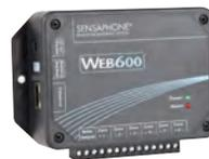
The WEB600 can monitor up to six external conditions including temperature from 109°F to 168°F, humidity, power failure and water detection. The device's built in web server hosts a web page where users can make programming changes, access status
