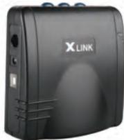
The XLink allows your Sensaphone to dial and receive calls using any cell phone with Bluetooth technology. It provides telephone service to a Sensaphone by placing a cell phone next to the device. The XLink will send all incoming calls to the Sensaphone and when the Sensaphone needs to dial out, the call will be seamlessly completed through the cell phone.
