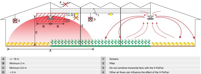
Е We recommend a max. installation height of 5 m for optimal results
