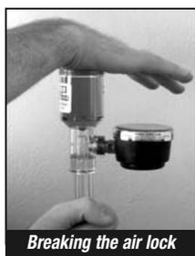
**Step 3 – Servicing** — Fill all IRROMETERS with a diluted solution of IRROMETER fluid (1 scant capful of concentrate to 1 gallon of water). Fill the IRROMETERS to the circle on the reservoir. Tap top of the IRROMETER with the palm of your hand to relieve any air lock. Take the vacuum pump and extract air from the instruments by pulling a vacuum of 80–85 cb (kPa) as registered on the gauge. Leave pump
