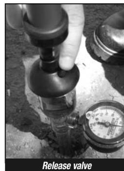
on the instrument for 10–15 seconds to allow air to rise and then release vacuum gently. Refill if necessary and replace cap until stopper comes in contact with bottom of the reservoir, then continue **tightening for 1/4 turn only.** Repeat pumping as above each time, after reading, for three or four times to improve sensitivity.
