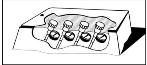
When used in pastures, IRROMETERS should be protected with a heavy concrete or steel pipe and the instruments installed at an angle so that the tips extend beyond the protective covering.
