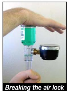
contact with reservoir bottom, then turn the cap 1/4 turn. Do NOT over tighten, this can damage the IRROMETER gauge or stopper.
