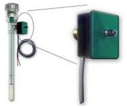
The IRROMETER RSU-C incorporates a pressure transducer and electronics in a potted waterproof housing. The RSU-C can be installed in the gauge port of any IRROMETER, thus converting the reading to a 4-20 ma loop current signal. It can be interfaced with a 4-20 ma loop current terminal or to an A/D card designed to read voltage. Excitation current required is 12 - 24 VDC.
