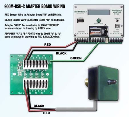
The 900M "RSU-C" Adapter board is used to adapt the RSU-C to the 900M series WATERMARK Monitor. An adapter board can be used to connect up to four "RSU-C" Transducers to the Monitor. Four "AA" size batteries (not included) are required to power the board.
