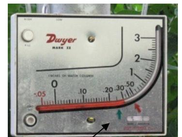
Our pressure gauge DWYER MARK III can take readings of air pressure between the roofs
