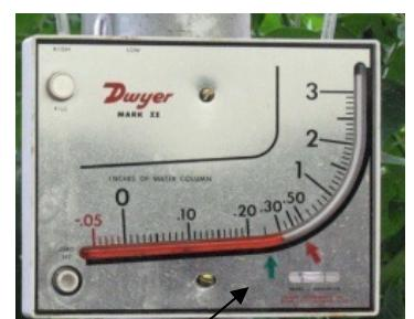
Our pressure gauge DWYER MARK III can take readings of air pressure between the roofs
